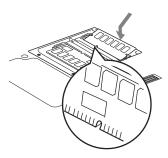
Figure 4-8. Installing a Second Memory Module
