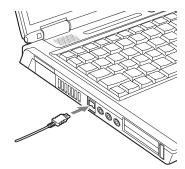
Figure 4-20. Connecting an IEEE 1394 Device
