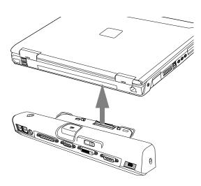
Figure 4-13. Attaching the Port Replicator
