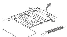
Figure 4-10. Removing a Memory Upgrade Module
