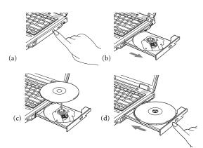
Figure 4-3. Loading/Ejecting Media
