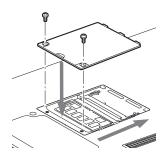
Figure 4-9. Replacing the Memory Compartment Cover
