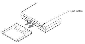
Figure 4-4.Loading/Ejecting a 3.5" Floppy Disk
