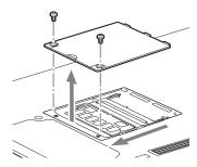
Figure 4-7. Opening the Memory Upgrade Compartment
