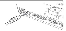
Figure 4-18. Connecting a PS/2 Device
