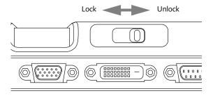
Figure 4-14. Locking the Port Replicator
