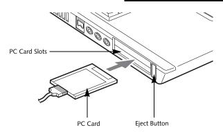
Figure 4-6. Installing/Removing PC Cards
