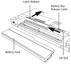
Figure 4-1. Removing a Battery
