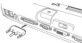
Figure 4-17. Connecting a Parallel Device to Port Replicator
