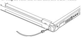
Figure 4-16. Connecting the LAN
