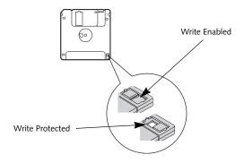
Figure 4-5. Floppy Disk Write Protect
