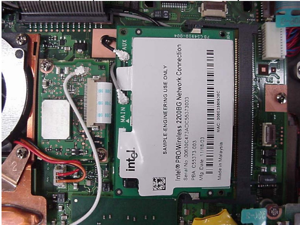
Calexico2 (WM3B2200BG) WLAN & Bluetooth – UGXZ5-102A – exploded view
