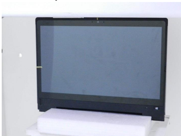
Edge1, Antenna Swivel 0, Test Separation 0 cm
