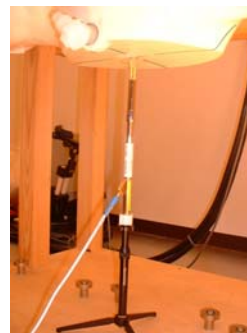
2450MHz System performance check setup
