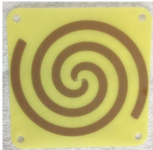
N-00241 Antenna Board – Side B:
