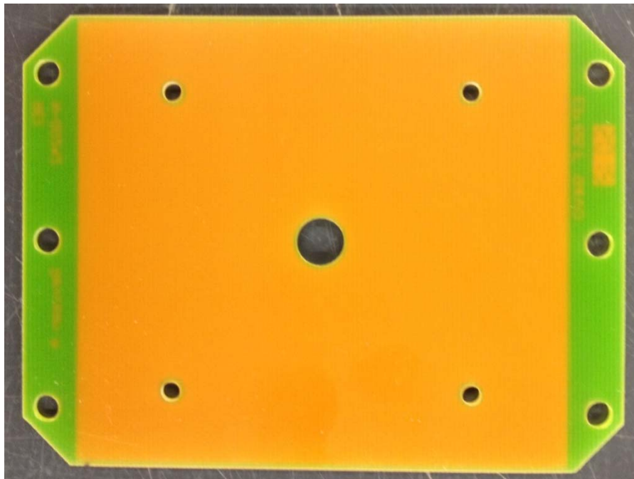
N-00242 Antenna Reflector – Side B:
