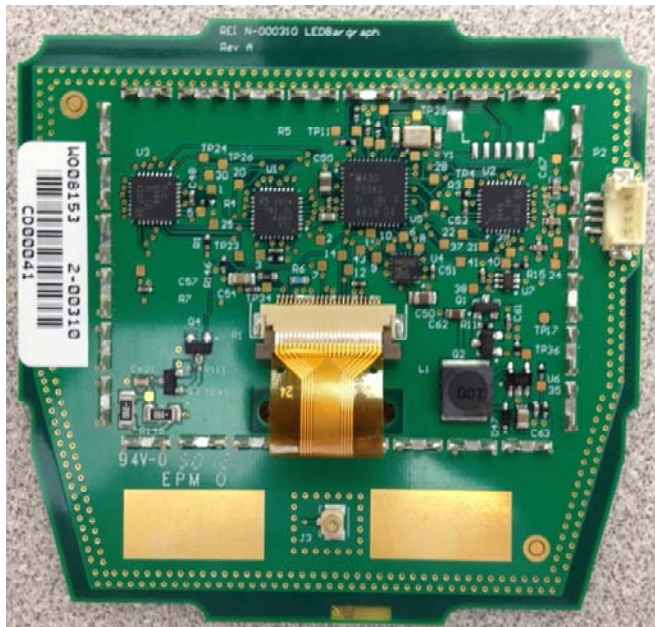
N-00310 LED Bargraph Board – Side A (without shields):
