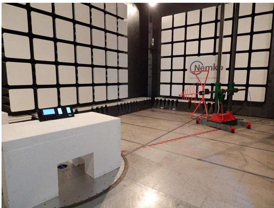
Figure 8.6-70: Radiated spurious (out-of-band) emissions setup photo – 30 to 1000 MHz
