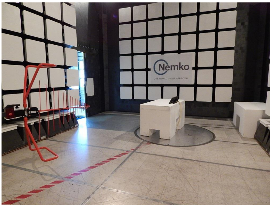
Figure 8.6-69: Radiated spurious (out-of-band) emissions setup photo – 30 to 1000 MHz
