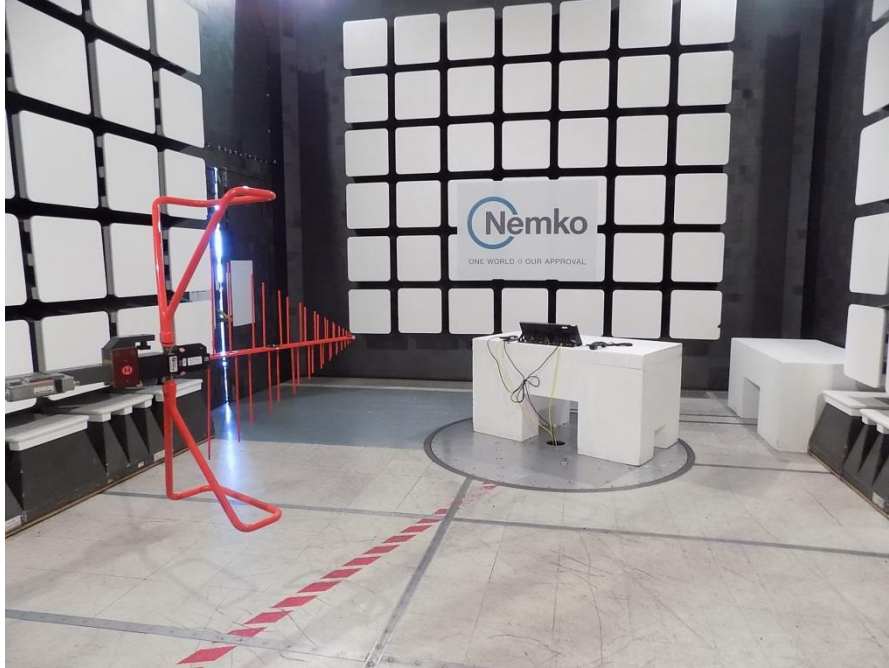
Figure 8.6-69: Radiated spurious (out-of-band) emissions setup photo – 30 to 1000 MHz
