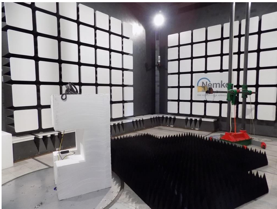
Figure 8.6-71: Radiated spurious (out-of-band) emissions setup photo – above 1 GHz
