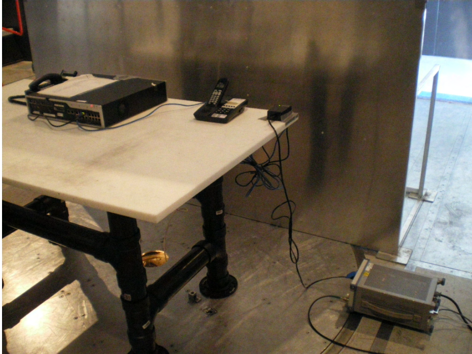
Photo 7.1-1: Conducted disturbance, front view
