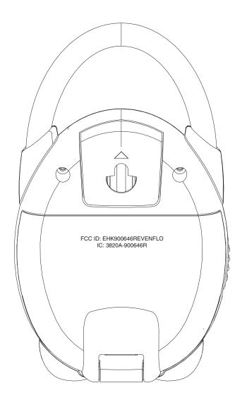
FCC ID & IC is engraved inside the battery compartment -All text to be molded, 0.16mm height
