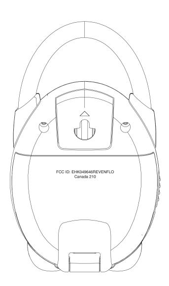
FCC ID & IC is engraved inside the battery compartment -All text to be molded, 0.16mm height
