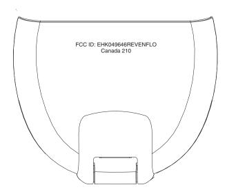
FCC ID & IC is engraved on the battery door -All text to be molded, 0.16mm height
