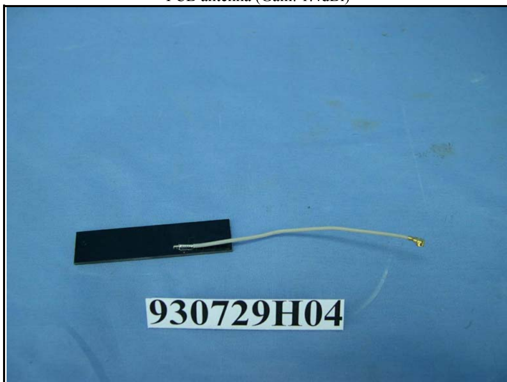
PCB antenna (Gain: 1.4dBi)
