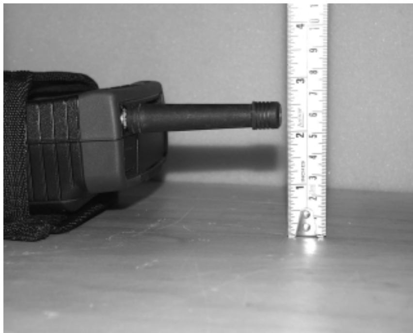
Photo 9: Shows detail of the distance to the antenna to the user with the 6100 within the pouch. 6100 facing forward.
