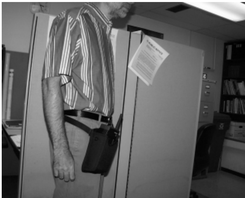
Photo 5: Shows the tablet computer within the pouch, antenna away from the operator.
