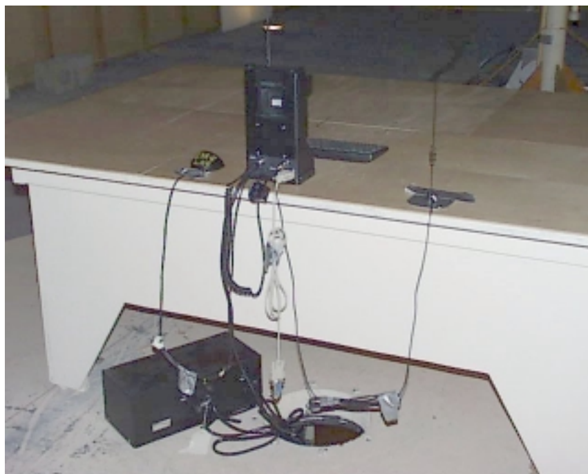
Photo 11: Shows the back view of the 6100 vehicle dock system with the external antenna.
