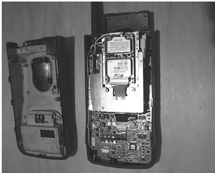
Photo 2: Shows the RIM902 radio within the 6100 showing the case back next to the opened unit.
