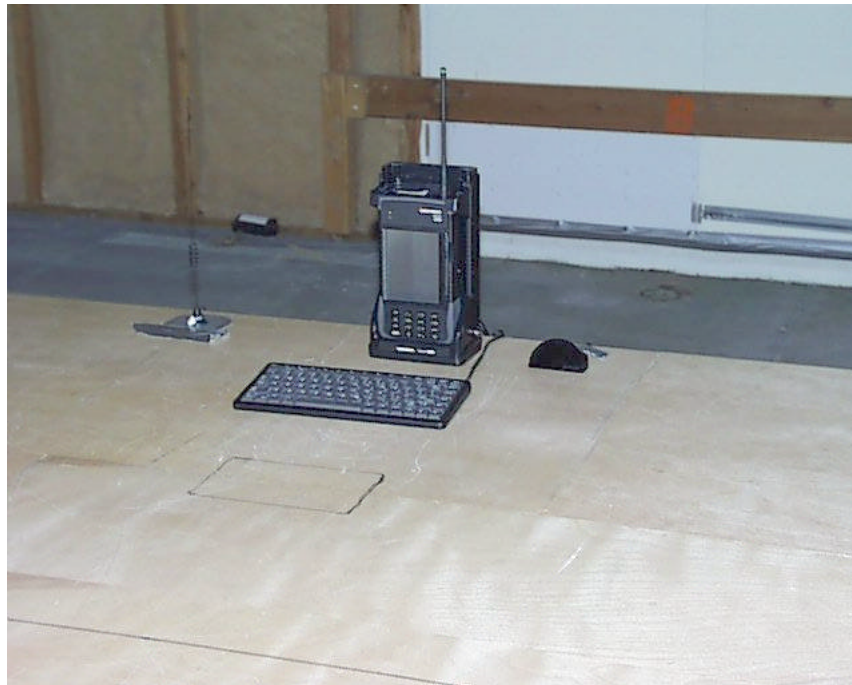
Photo 11: Shows the front view of the 6100 vehicle dock system with the external antenna.
