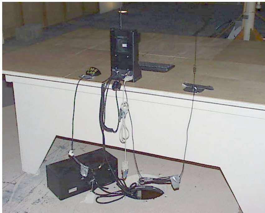
Photo 12: Shows the back view of the 6100 vehicle dock system with the external antenna.
