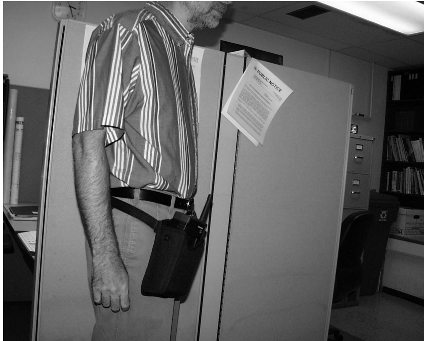
Photo 5: Shows the 6100 tablet computer within the pouch, antenna away from the operator.
