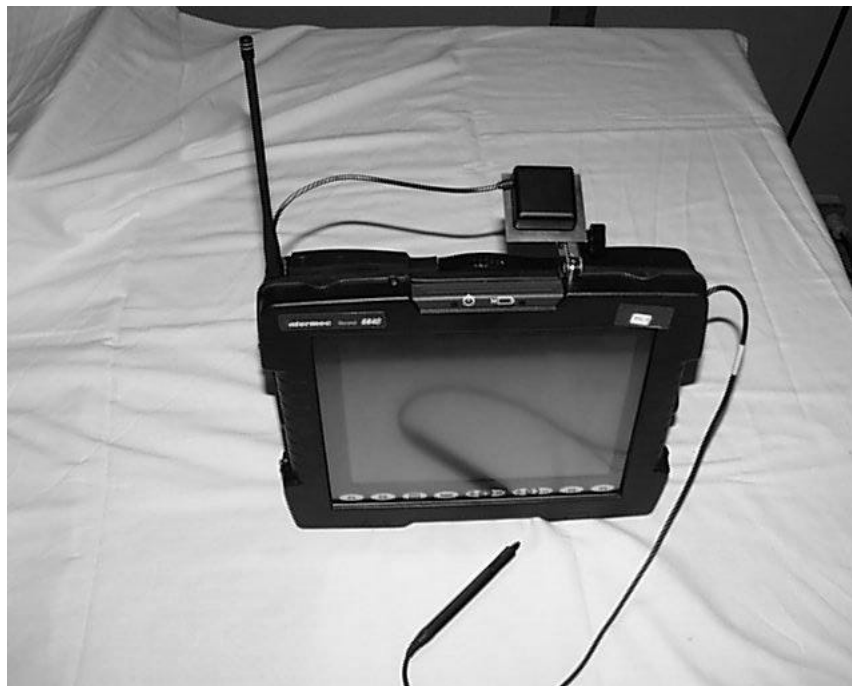
Photo 12: Shows the top view of the 6600, this unit also has the optional GPS antenna.
