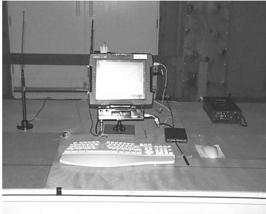
Photo 13: Shows the 6600 within the vehicle dock and the remote antenna connected.
