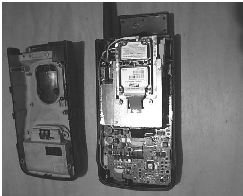
Photo 2: Shows the RIM802 radio within the 6100 showing the case back next to the opened unit.
