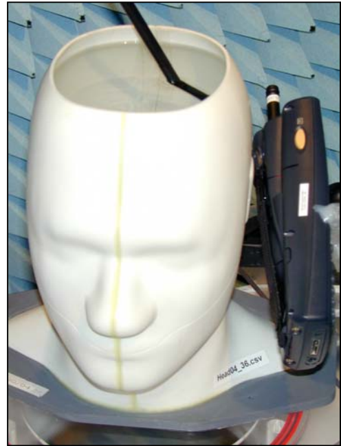
Figure 64. Positional photograph of the Intermec 700C Handset in the Left-Hand 15 degree position
