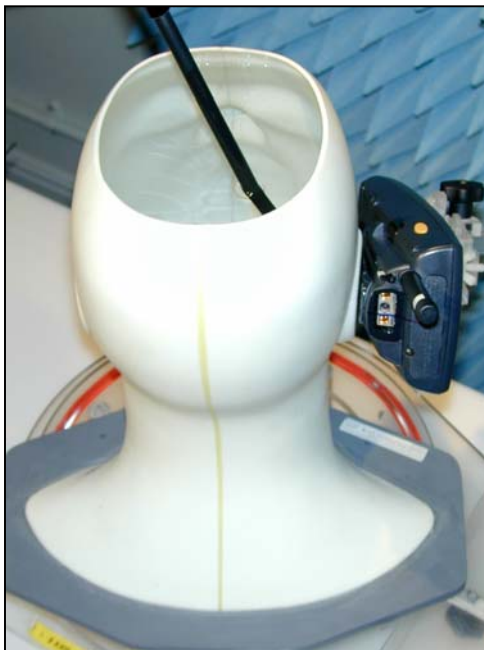
Figure 65. Positional photograph of the Intermec 700C Handset in the Right-Hand Cheek position
