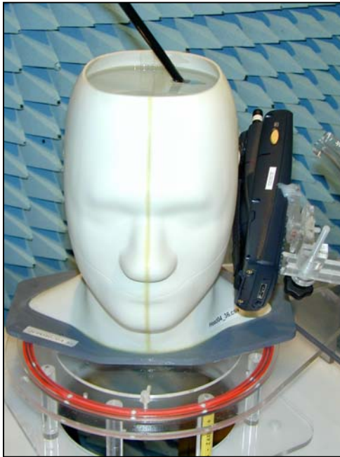
Figure 63. Positional photograph of the Intermec 700C Handset in the Left-Hand Cheek position
