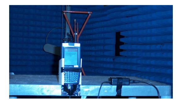
700C - Radiated Emissions Test Set-up
