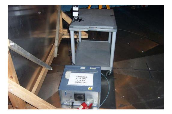
700C - Conducted Emissions Test Setup
