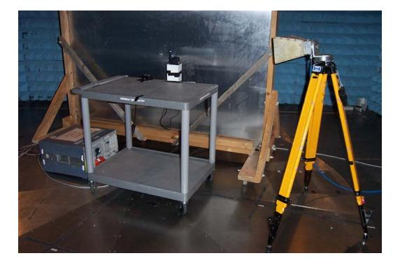
700C – Conducted Emissions Test Setup
