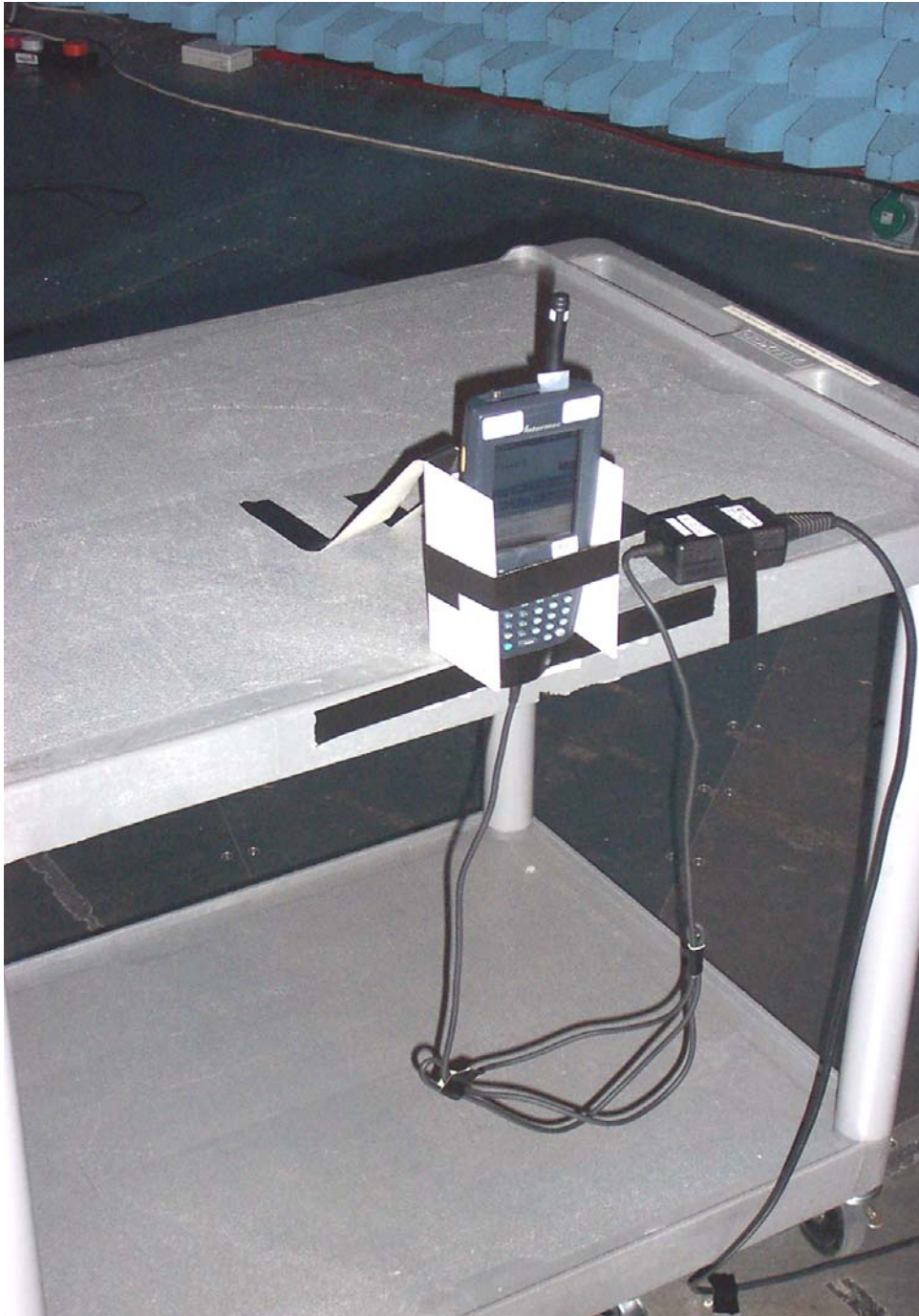
Effective Radiated Power Set Up Photograph
