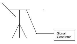
The spectrum analyzer is monitored to verify that the output of the signal generator produces a signal equal in amplitude to a previously measured spurious emission.
