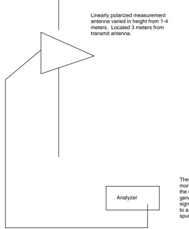
During field strength measurements, the amplitude and frequency of the highest emissions are noted. The transmitter is then replaced with a ½ wave dipole (at the same height) that is successively tuned to each of the highest spurious emissions. A signal generator is connected to the dipole (horn antenna for frequencies above 1 GHz), and its output is adjusted to match the level previously noted for each frequency.
