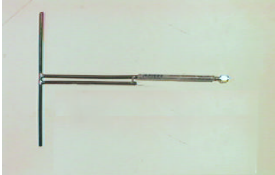
Reference Dipole Antenna Used for the Measurement
