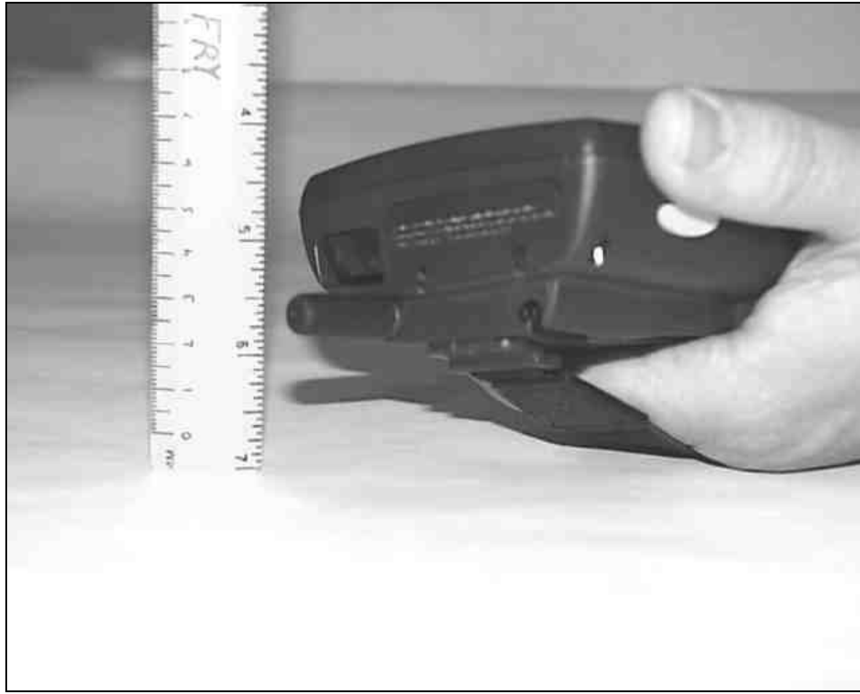
Photo 3: Shows the antenna distance to the user body with the unit operated within the hand.
