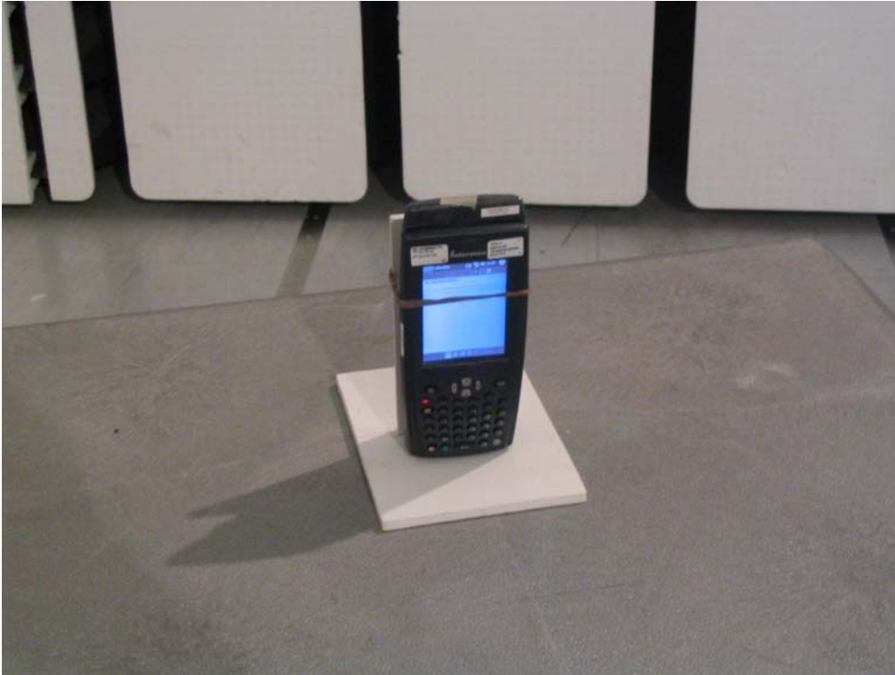
Radiated Emissions Test Setup
