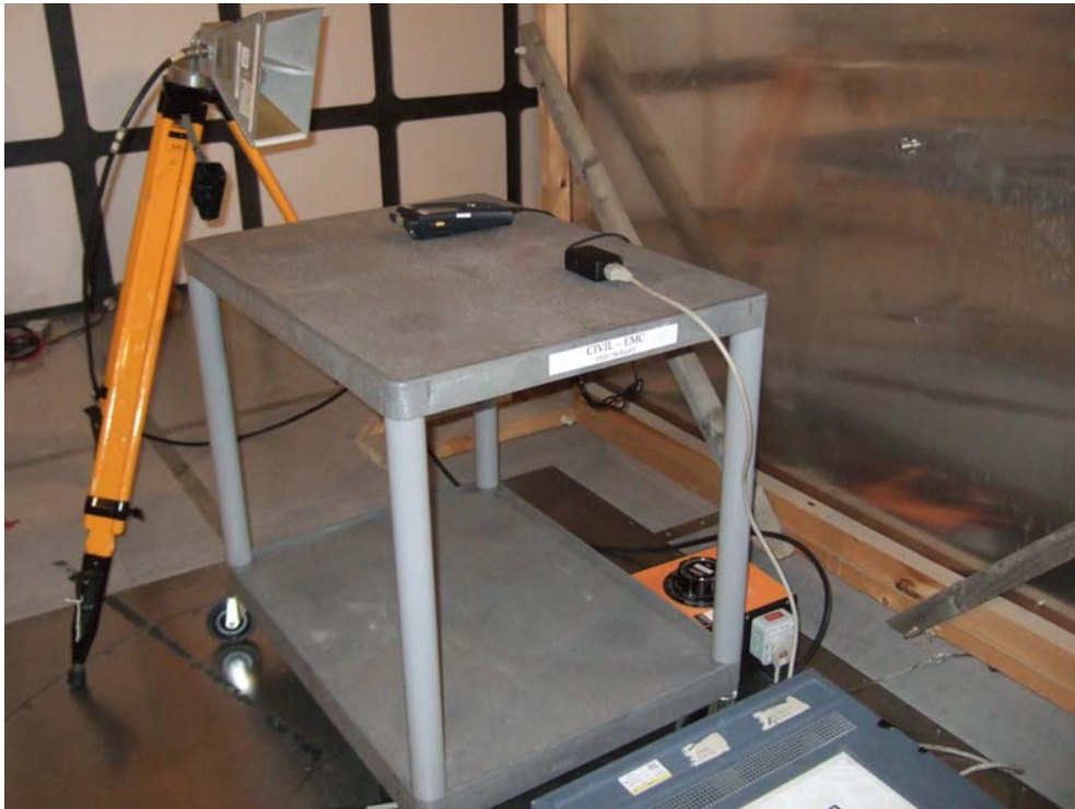
Conducted Emissions Setup
