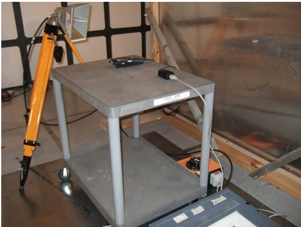
Conducted Emissions Setup
