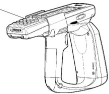
**3** Attach the two retaining screws. Ensure that they go straight into the mobile computer openings.
