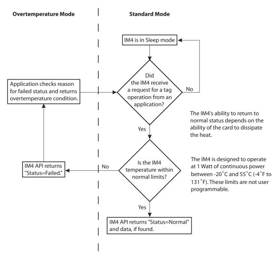
This flow chart illustrates how the IM4 operates in Overtemperature mode and in Standard mode.
