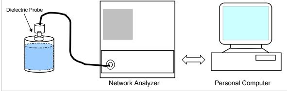
Set-up for liquid parameters check
