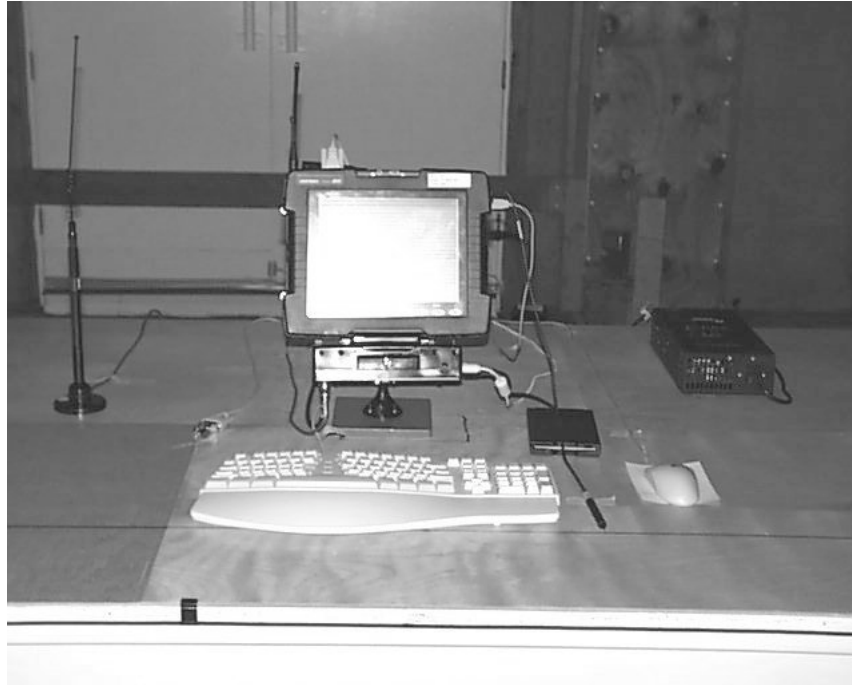
Photo 7: Shows the 6600 within the vehicle dock and the remote antenna connected.
