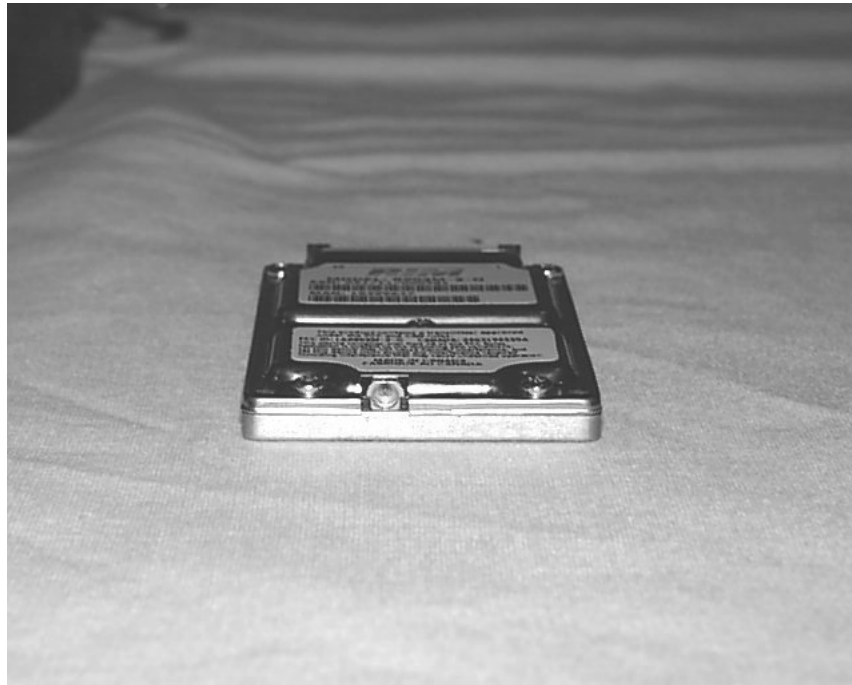
Photo 5: Shows the bottom view of the radio module and antenna connector.
