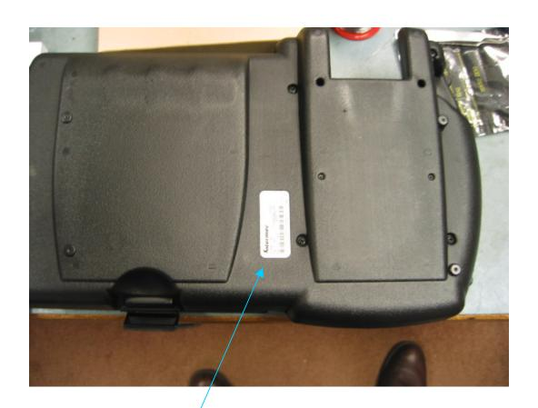
FCC ID Label Location on Bottom of PW40 Printer
