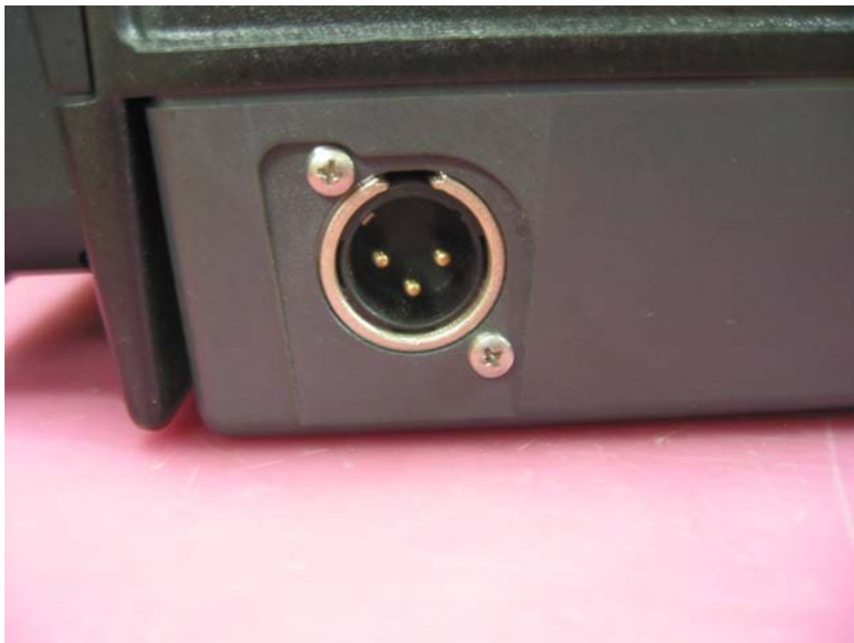
Close-up of DC Power Input
