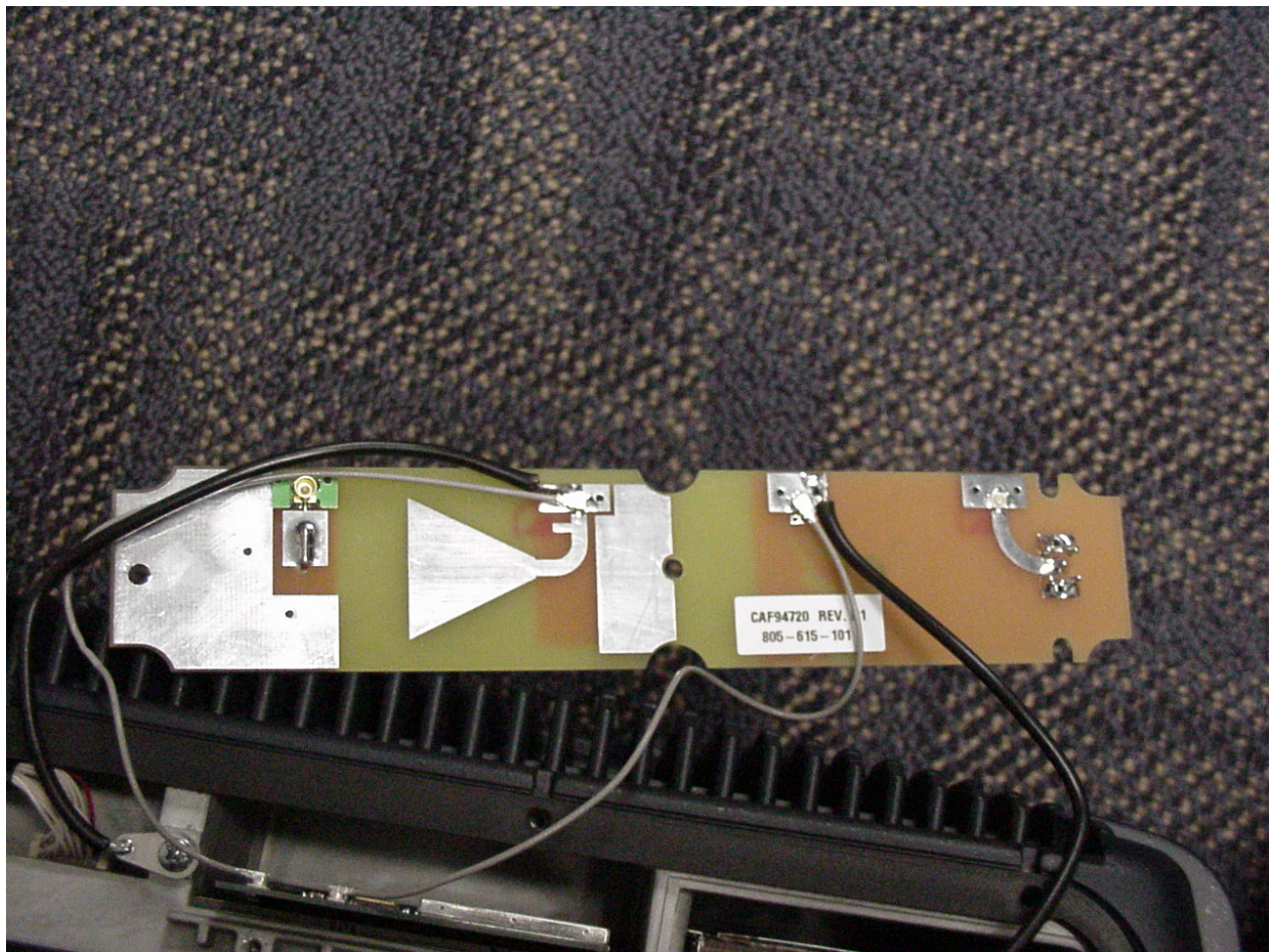
CV60 Showing Bottom of 802MIAG Antenna Board
