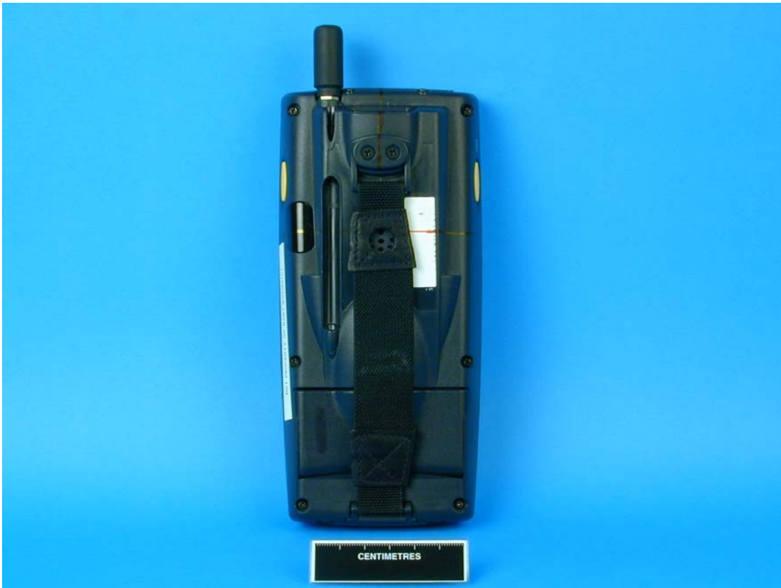
Figure 4. Rear View of the Intermec Handheld Computer Terminal, 700C-SMC45, Showing the vertical and horizontal lines (marked in red and with the carrying strap in position) used for the alignment procedure as defined in Draft IEEE Std1528. – December 29, 2002
