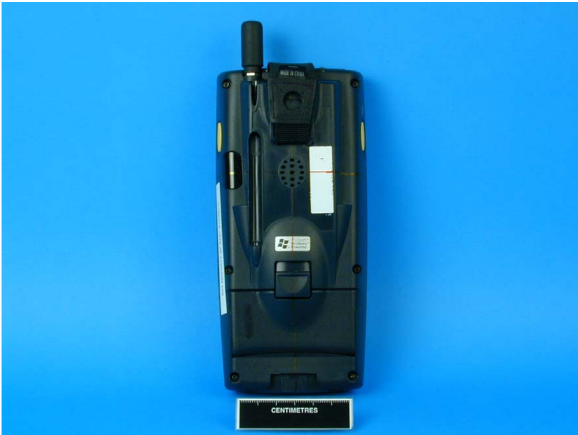
Figure 5. Rear View of the Intermec Handheld Computer Terminal, 700C-SMC45, Showing the vertical and horizontal lines (marked in red and with the carrying strap moved out of position) used for the alignment procedure as defined in Draft IEEE Std1528. – December 29, 2002
