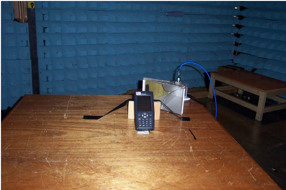
The photograph below shows the EUT configuration during Radiated Emission testing.
