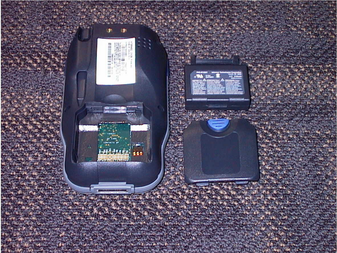
Back of CN2B with Battery Removed
