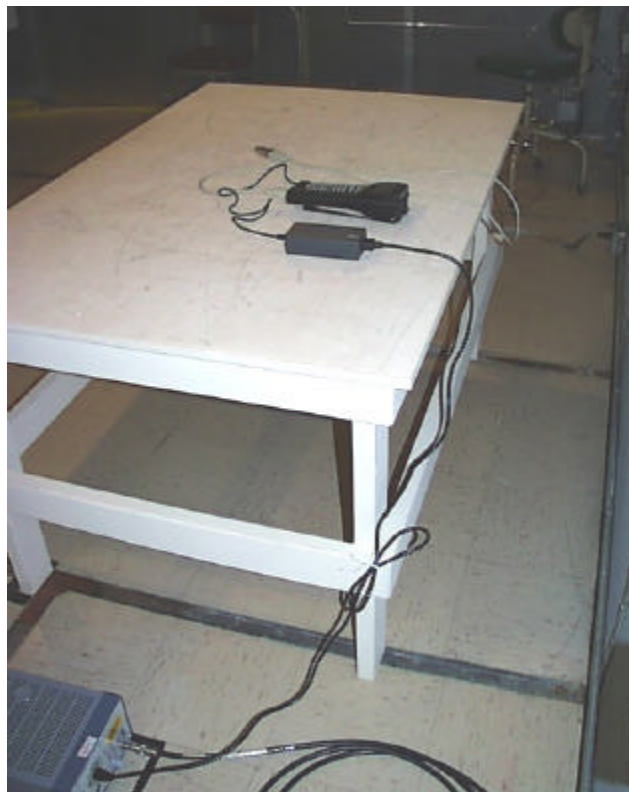
Photo 16: Shows the 2126 within 6400 during maximum AC conducted emissuion testing.
