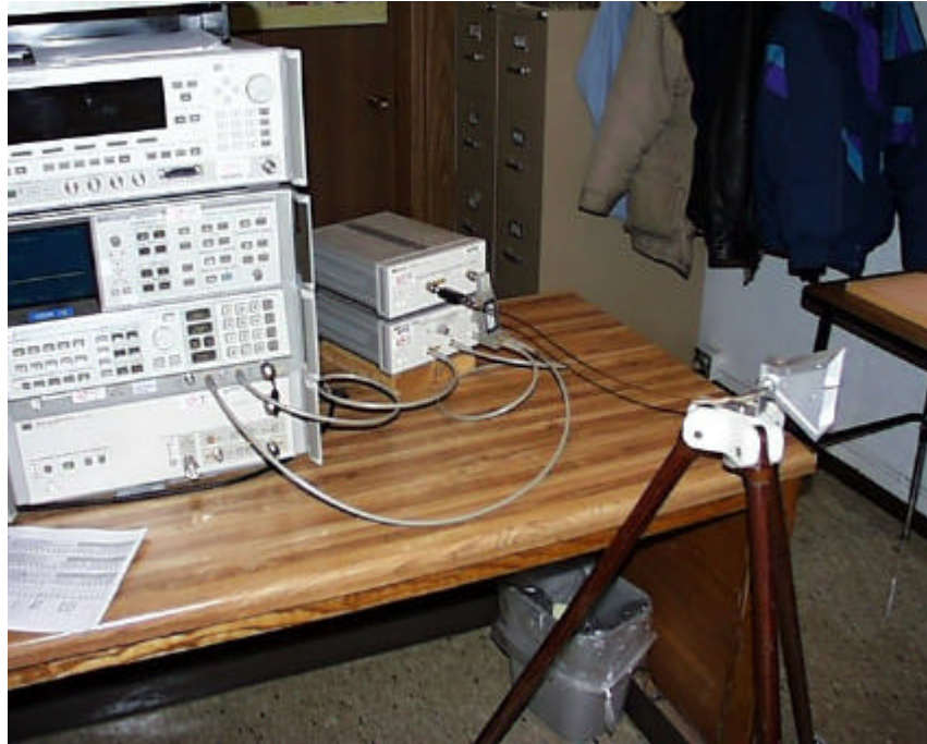
Photo 9: Shows the measurement setup used during radiated testing above 18 GHz.
