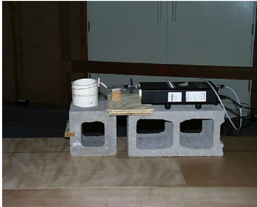
Photo 1: Shows the horizontal placement of the 2126 module on the OATS with Radial antenna.
