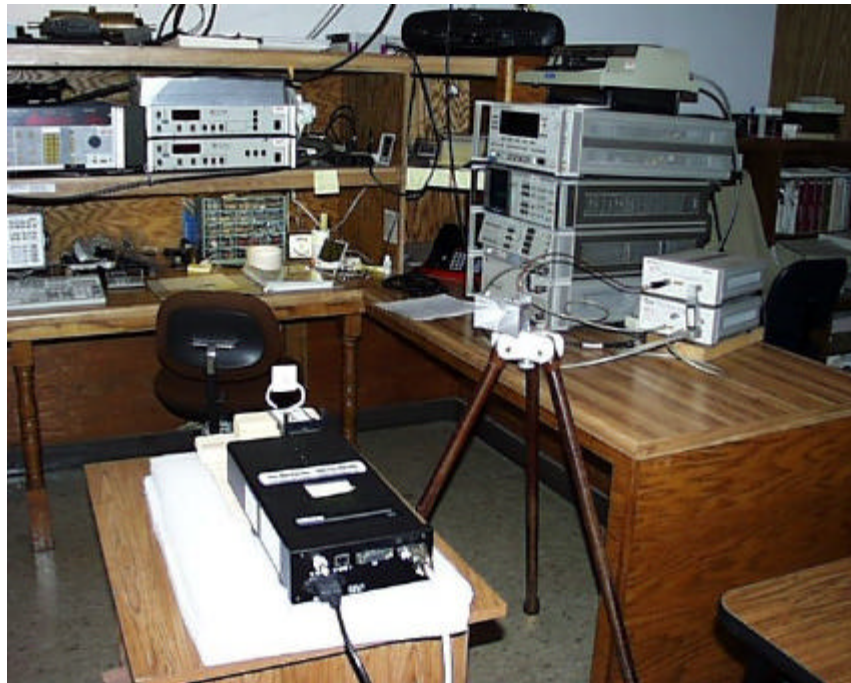
Photo 10: Shows horizontal placement of the 2126 radio with Radial antenna >18 GHz testing.
