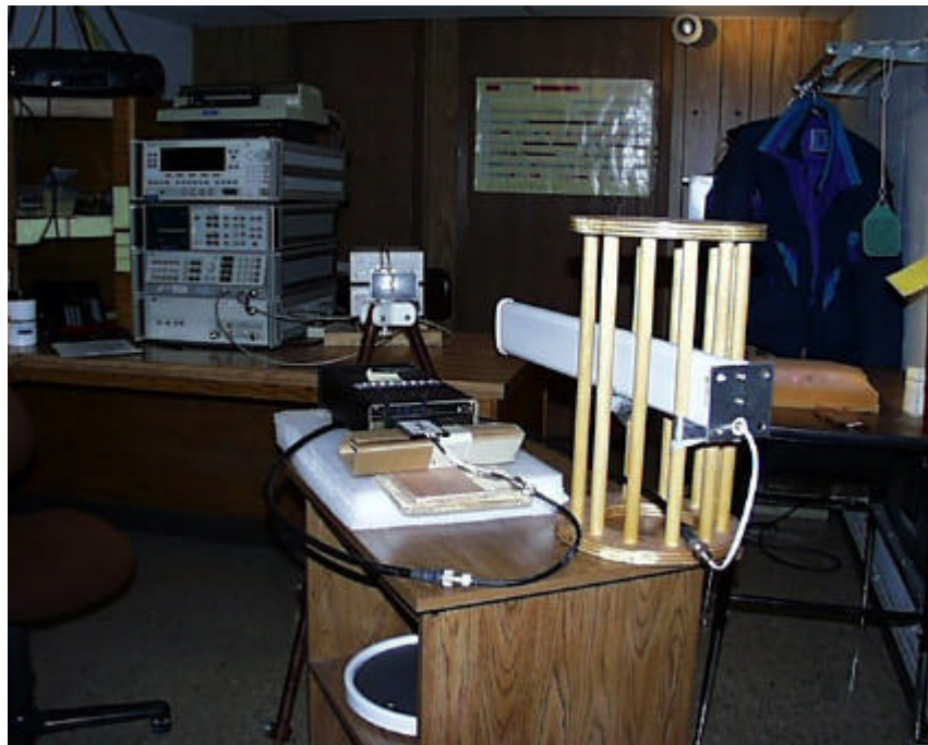
Photo 14: Shows placement of the 2126 radio with Cushcraft antenna >18 GHz testing.
