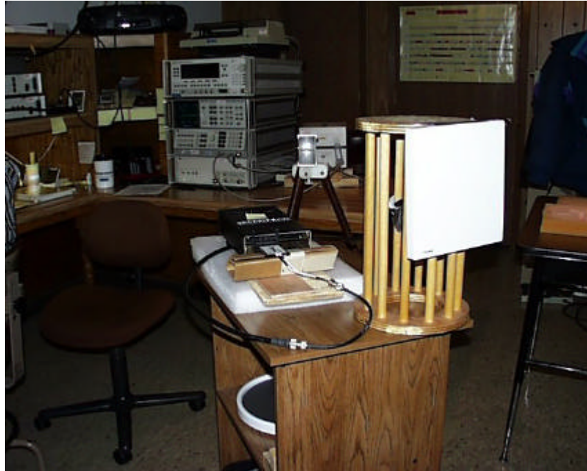
Photo 14: Shows placement of the 2126 radio with Cushcraft antenna >18 GHz testing.
