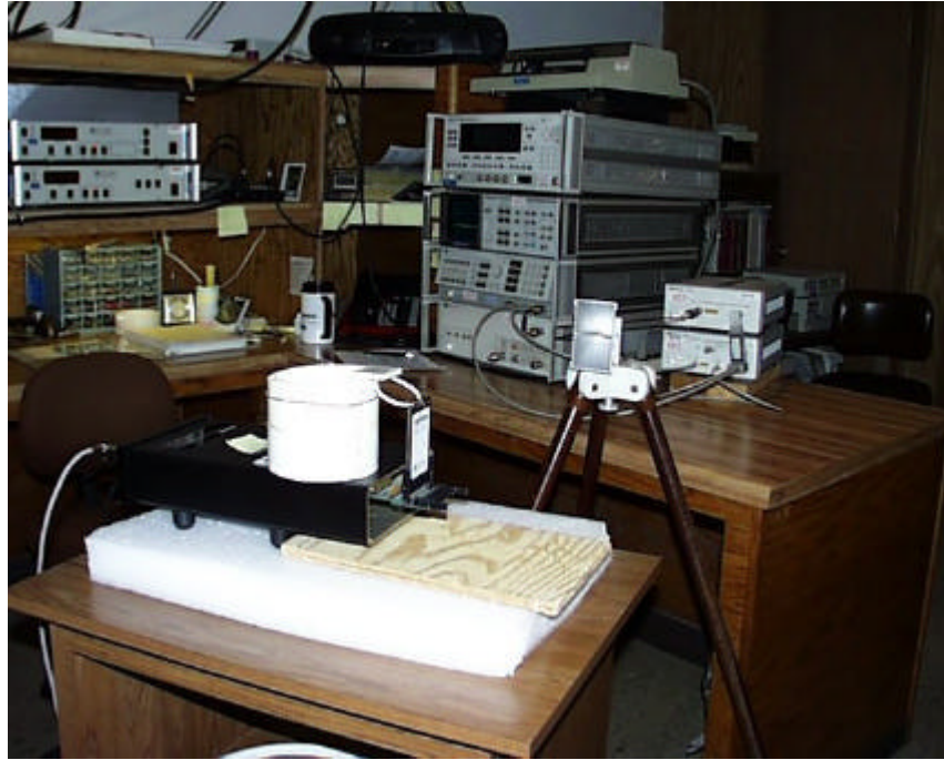
Photo 11: Shows vertical placement of the 2126 radio with Radial antenna >18 GHz testing.
