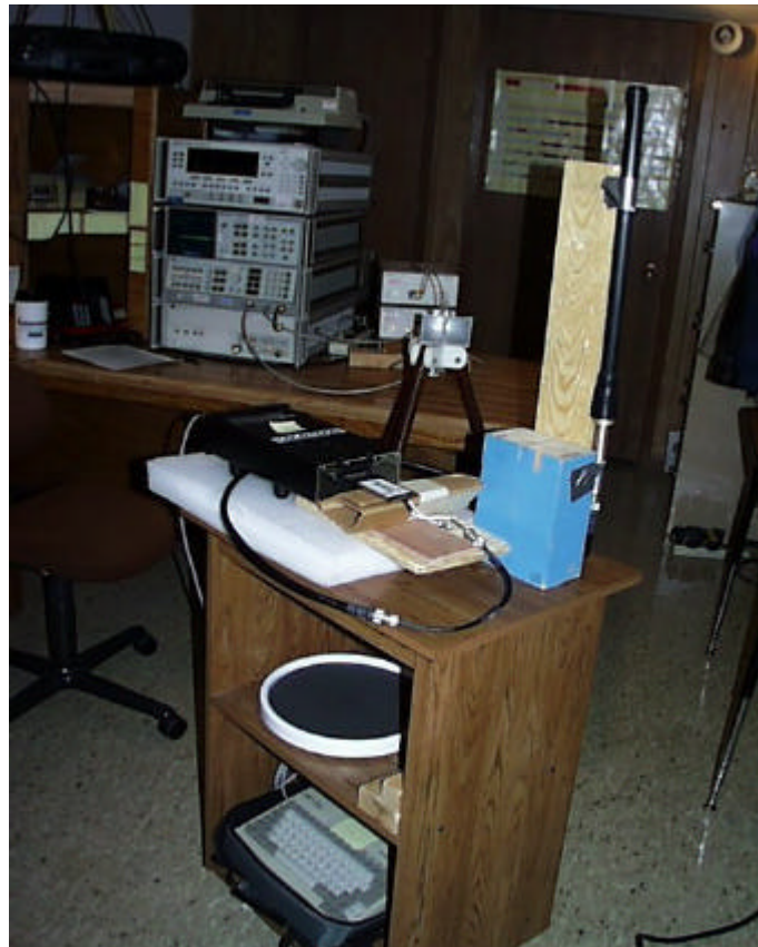
Photo 12: Shows placement of the 2126 radio with Mobile Mark antenna >18 GHz testing.
