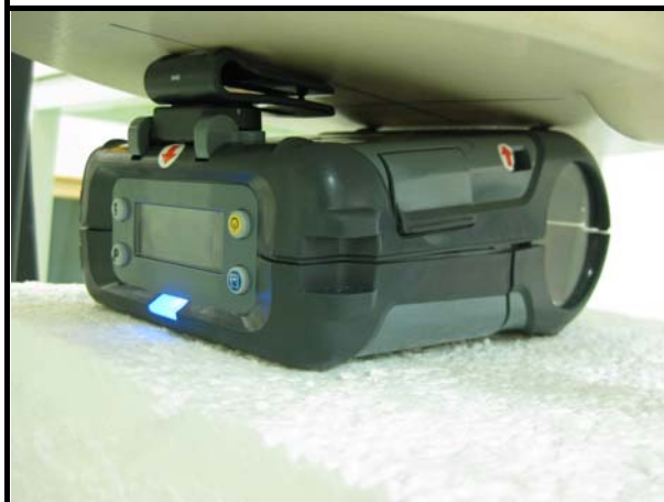
B. The bottom of the EUT face to the phantom with 0mm-separation distance.
