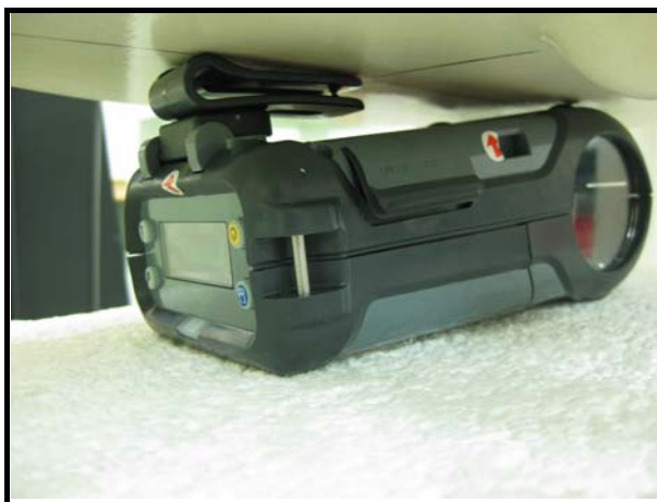
A. The bottom of the EUT face to the phantom with 0mm-separation distance.
