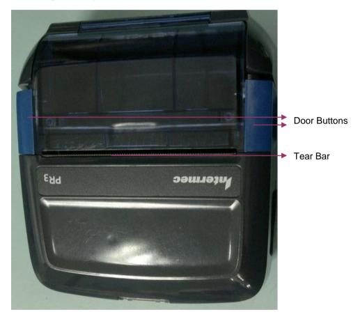
Figure 1: A PR3 Printer (Top View)
