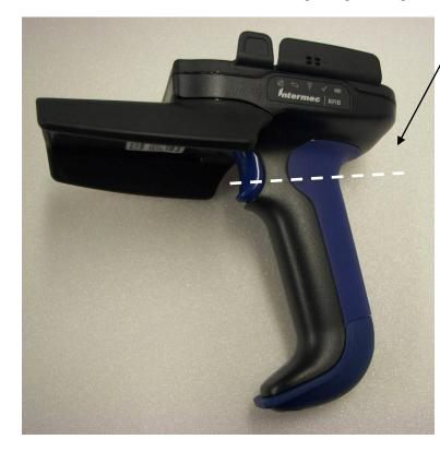
The battery was removed from handle, then the handle was cut along the dotted line so it could be placed against the flat phantom at the correct distance from the hand placement
