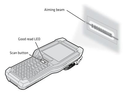
When the CK3 successfully reads a bar code label, you hear a high beep, and the Good Read LED turns on briefly.
