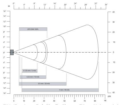
**EV12+ Linear Imager Typical Reading Distances:** This graphic does not include the 0.12 cm (0.05 in) setback for the CK3.
