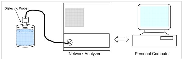
Set-up for liquid parameters check
