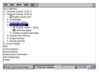
**6** Go to **Scanner Settings** > **Scanner model** and select your scanner from the list.
