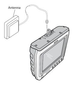
Attaching an External Antenna
