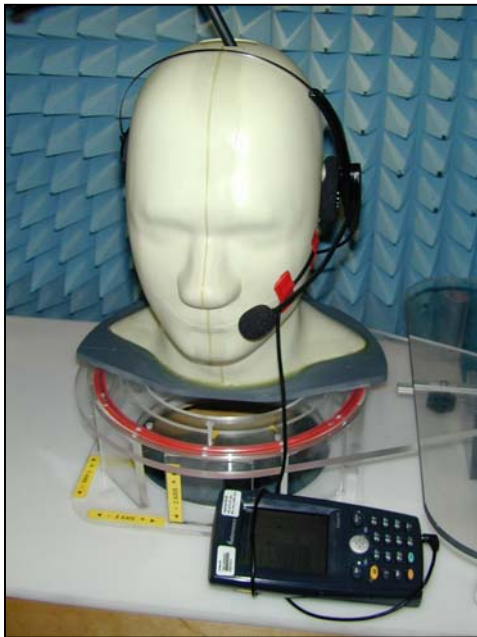
Figure 34. Positional photograph of the Pocket PC Model, 730 using a 'Industry Standard' Headset against the SAM Phantom.
