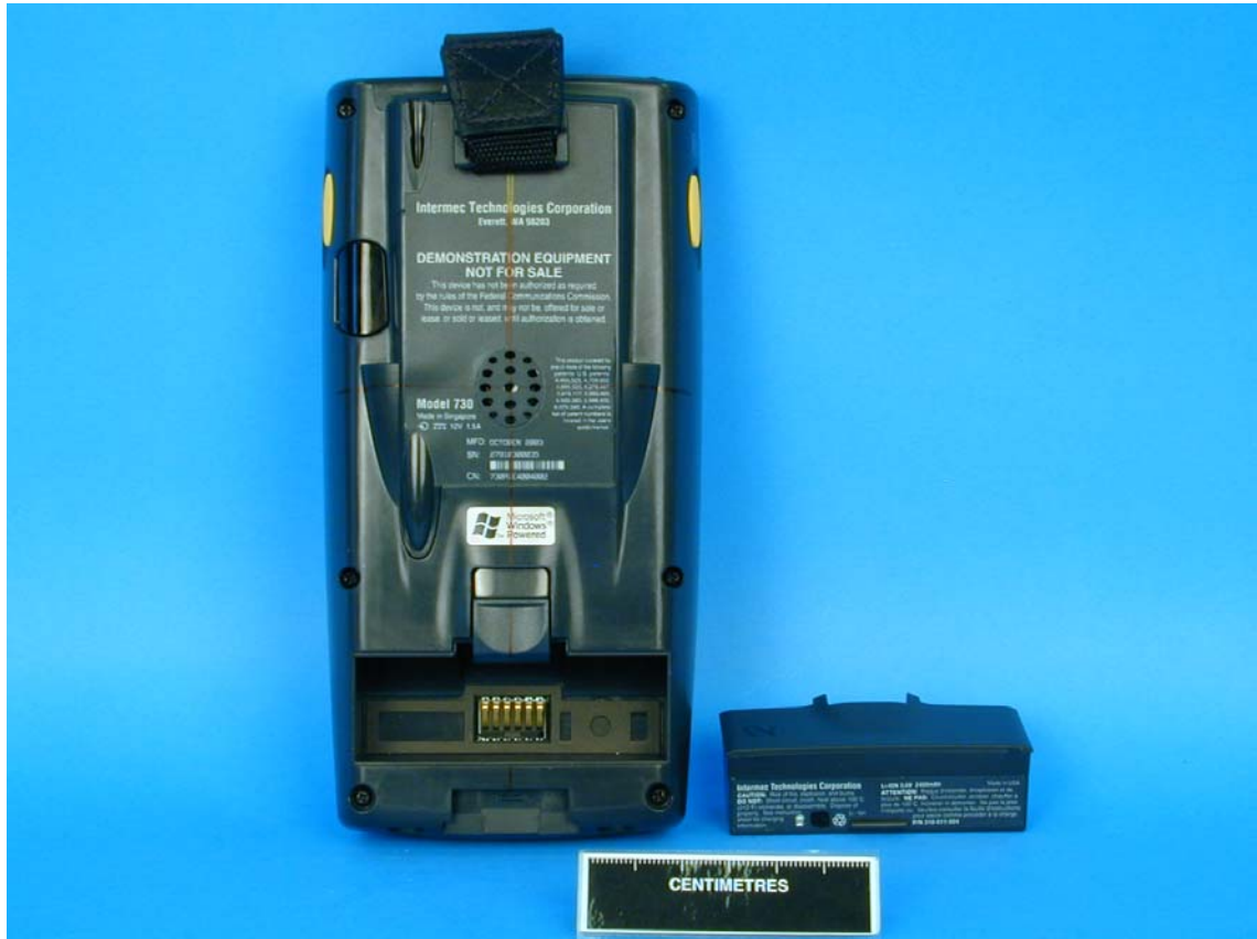
Figure 43. Rear view of the Intermec Technologies Corporation Pocket PC Model 730. With the battery removed
