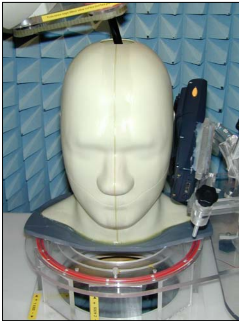
Figure 30. Positional photograph of the Pocket PC Model, 730 in the left-hand Cheek Position
