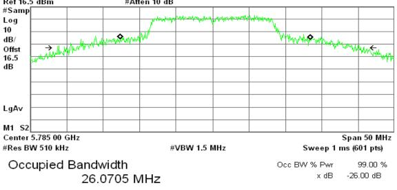
Transmit Freq Error371.120 kHzx dB Bandwidth42.125 MHz\*
