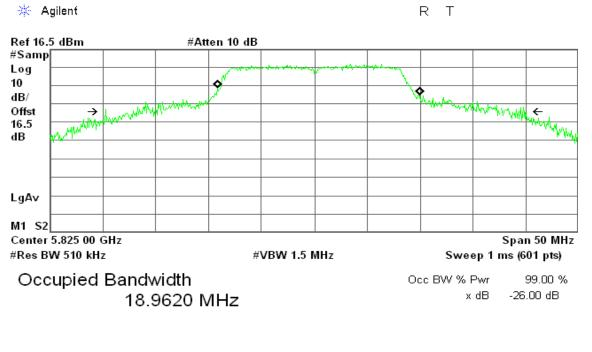
Transmit Freq Error394.990 kHzx dB Bandwidth39.498 MHz\*
