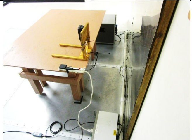
AC Conducted Emission (Rear View)
