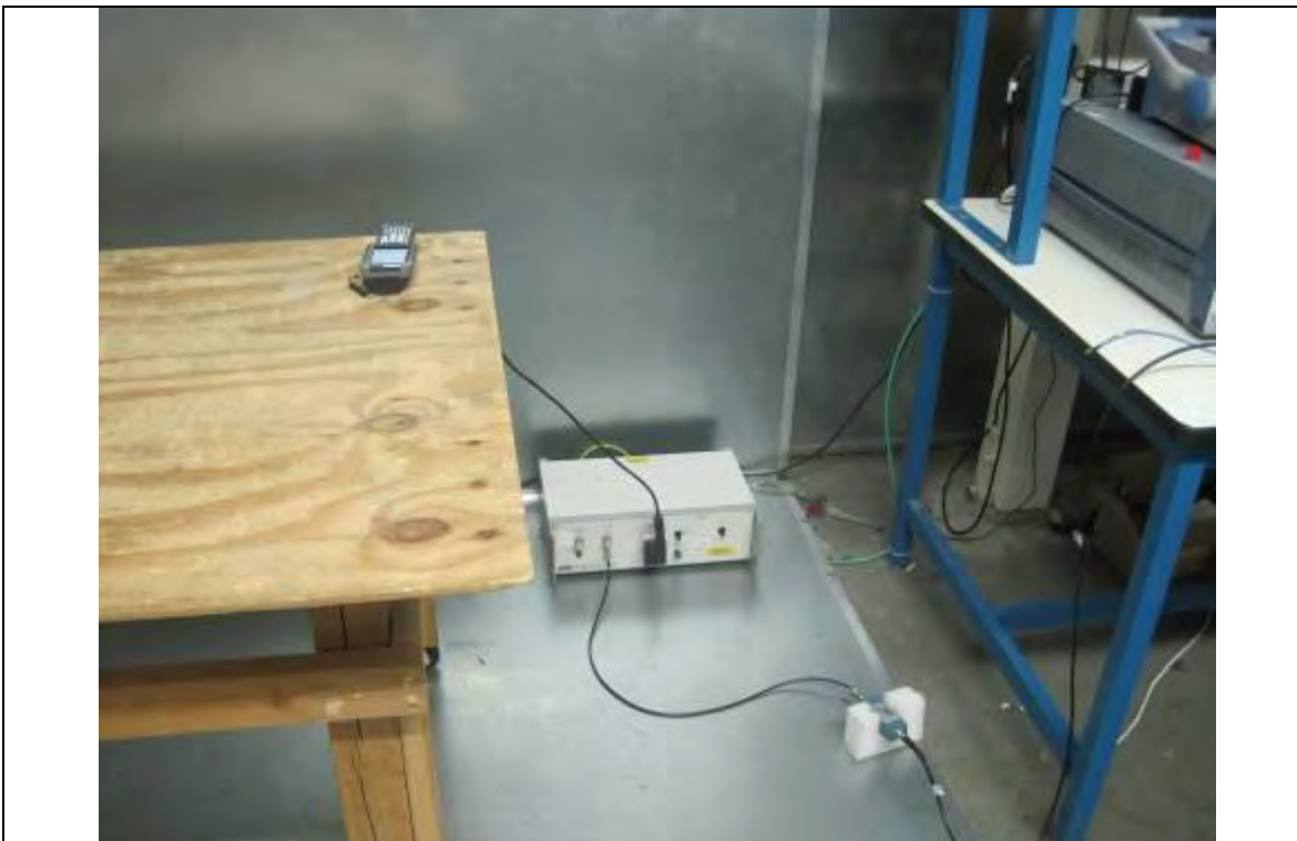
Conducted Emission Test Setup – Front View
