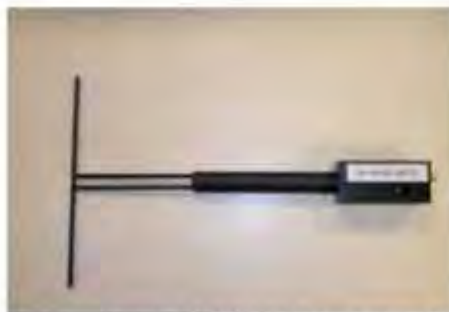
Figure 1 – Satimo COMOSAR Validation Dipole
