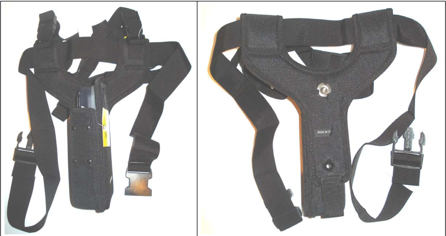
DUT with Holster & Y-Belt Body-worn accessory – Left Side of DUT facing user's body (antenna side closest to user)
