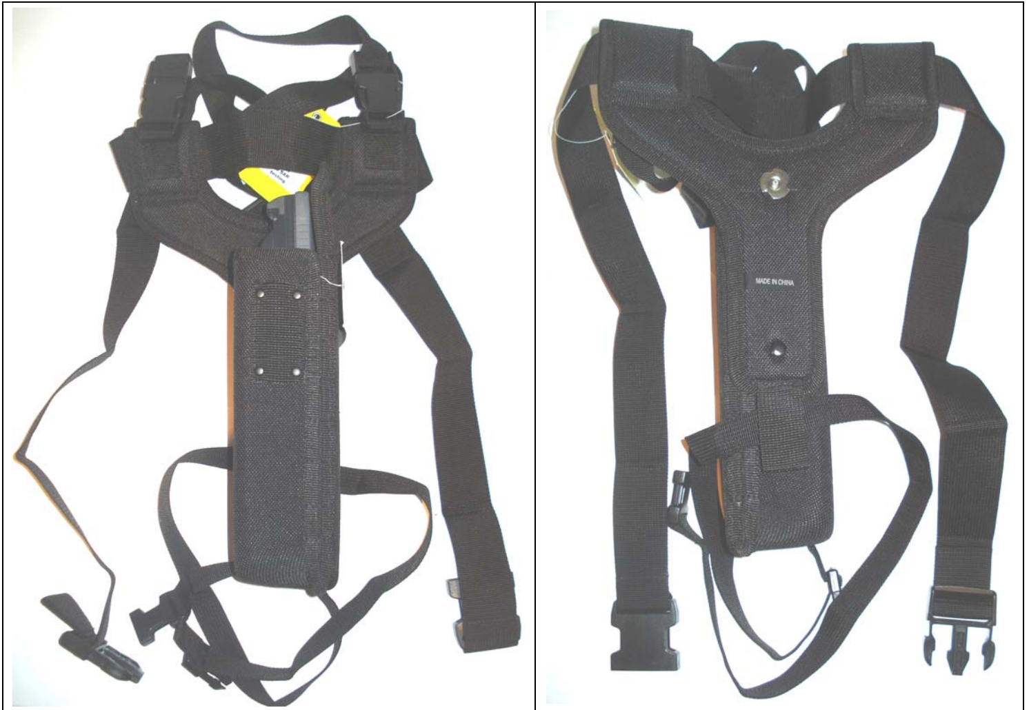
DUT with Holster & Y-Belt Body-worn accessory – Left Side of DUT facing user's body (antenna side closest to user)
