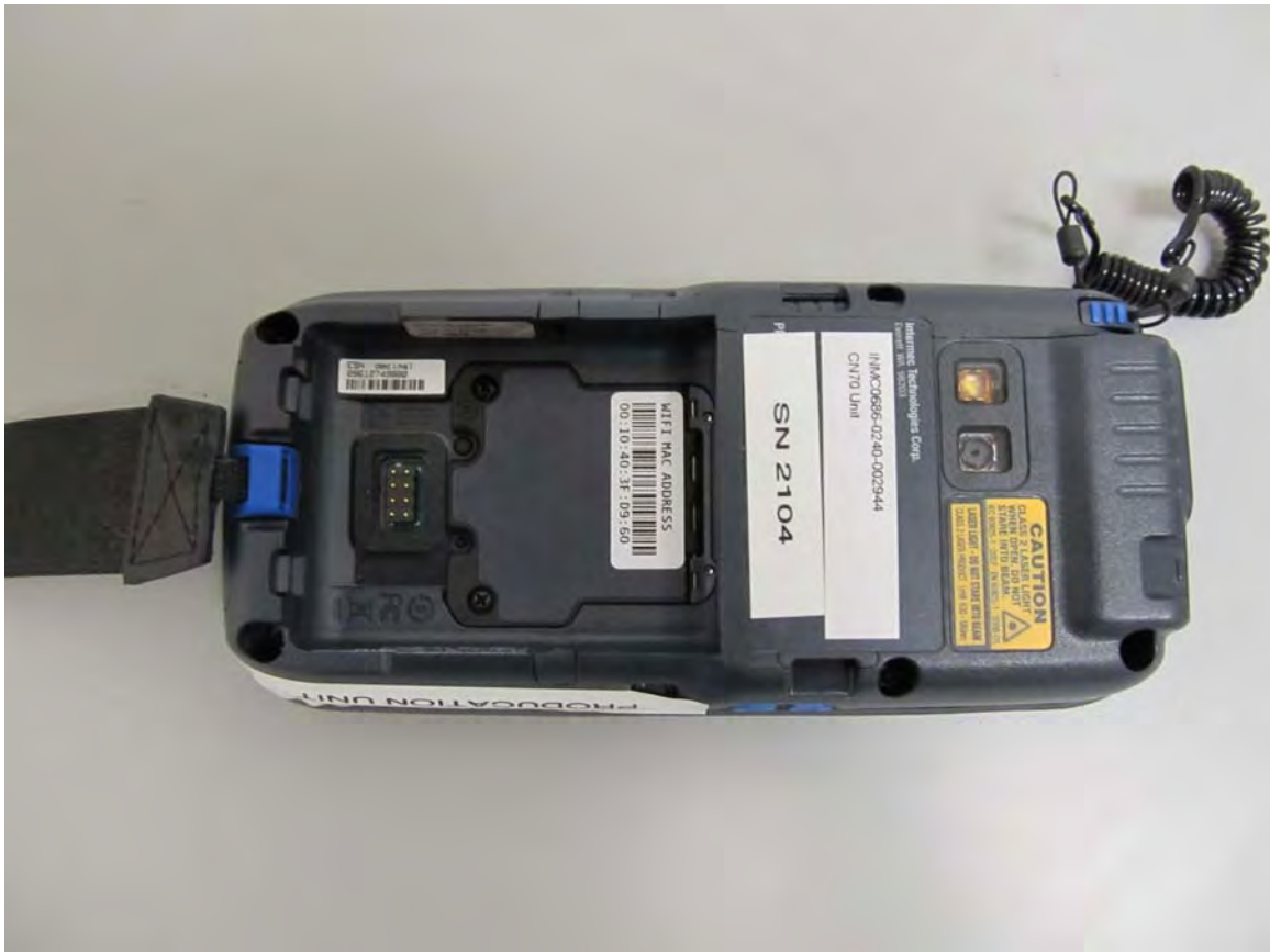
Back side – battery cover removed
